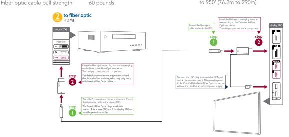
Celerity Technologies' Fiber Optic Plug terminating each end of the Celerity Fiber Optic HDMI cable supports proprietary technology for HDMI over Celerity Fiber Optic cable. While the plug may appear similar to that of micro-HDMI or mini-USB, it does not support any technical attributes of either connector. The Celerity fiber optic plug supports only proprietary Celerity technology and is connected to the Celerity Fiber Optic HDMI connector according to the user guide
